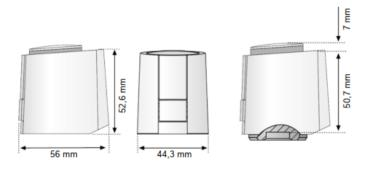
Standard with plug-in cable AXT301F100/102
