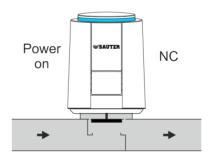
On delivery, the first-open function is active, which means the actuator is in the open state when deenergised. This means it can be installed without applying much force and the valve remains open. This allows heating operation in the construction phase. The first-open function is deactivated by applying supply voltage for at least 6 minutes and the actuator is fully operational.
