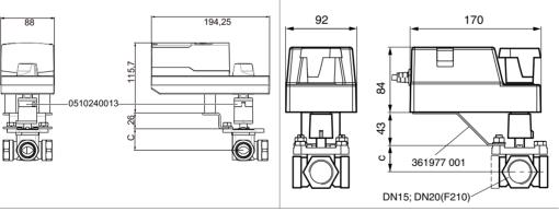
M4R 4-way control valves with actuator ASM 105/115
