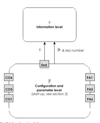
PA1/CO1: Rk1 (heating circuit 1) PA5/CO5: System-wide parameters PA6/CO6 Modbus communication
