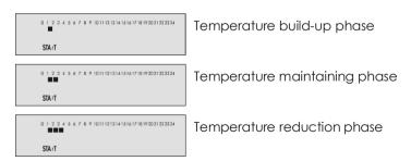
The drying process has been successfully completed when the additional icon in the flow temperature display goes out after the last phase.
