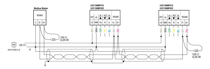
The max. admissible bus length depends on the cable type used and the correct termination with terminating resistors. In general, a 2-wire shielded cable with twisted wire pairs must be used. Use of one of the following cable types is recommended:
