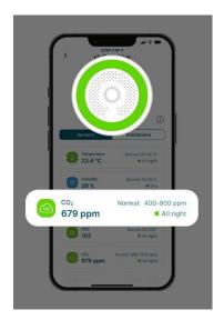
The app makes it easy to commission the smart sensor and integrate it in the Bluetooth network. Real-time CO<sub>2</sub> readings now complement the sensor mix for VOC, temperature, humidity, brightness, presence and sound level.
