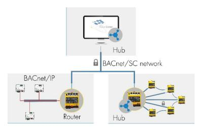
With BACnet/SC-capable software and hardware from SAUTER, existing BACnet installations can be BACnet/SC encrypted.
