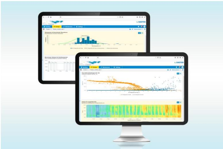
With the display of scatter and carpet plots, operating pattern and setpoint deviations can be detected immediately.
