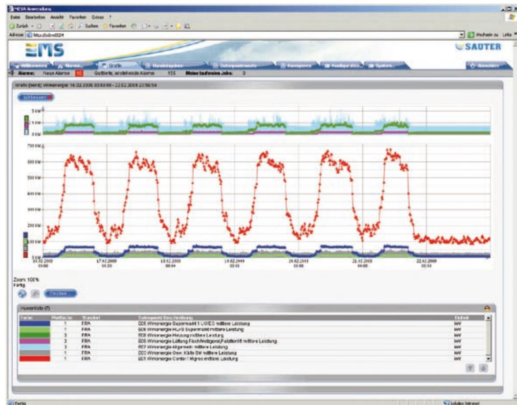
SAUTER EMS provides a continuous dynamic display of the entire energy consumption within an integrated system, as well as consumption figures for individual buildings, sections of buildings or equipment systems.
