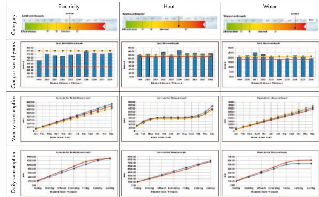
SAUTER EMS allows comparisons of consumption at any time between current and previous periods, and it also tracks the development of energy efficiency.
