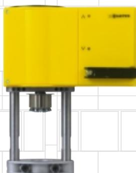
Actuator with 2500 N pushing force without spring return, and 2000 N pushing force with spring return; mechanical manual adjustment; automatic drive-valve coupling.
