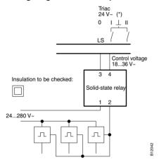
Constant actuators for unit valves with AXS positioner.
