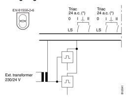
Supplying power to the actuators via semiconductor relay. (The number of actuators is limited by the output of the semiconductor relay.) Semiconductor relays can be ordered from stock at SRF.
