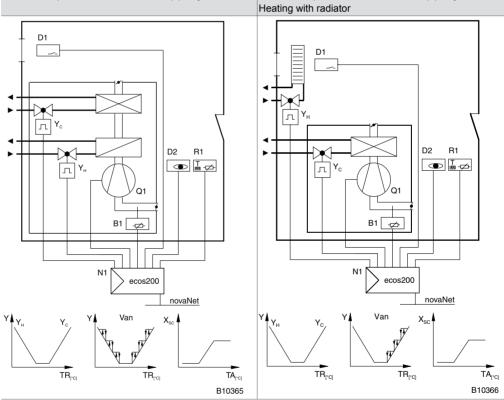
Fan coil temperature controller with 4-pipe system Heating with radiator
