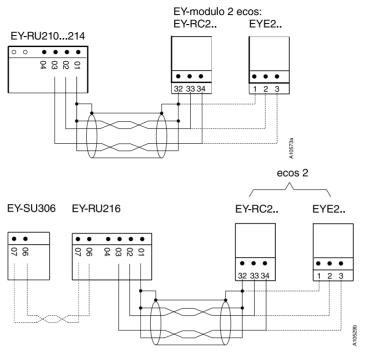
The resistance to interference of the transmission between the operating unit and the ecos is increased by using twisted connecting cables.
