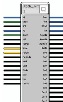
The ecoUnit 1 room operating units behave in a similar way to the wired room operating units. The data received from the transmitters is represented on the ROOM\_UNIT firmware module in the ecos 5. Window contacts and switches are evaluated using the (Sw) 1...12 buttons of the ROOM\_UNIT module.
