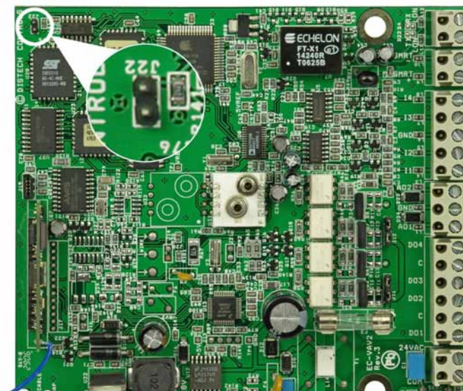
Fig. 24 Memory erase jumper location (J22) on ecos416
